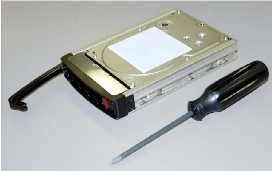
**Figure E-2** Hard disk drive in a carrier
